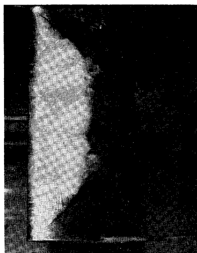
Fig. 9 Extent of cavitation at four different cavitation numbers for \alpha = 8^\circ , \Lambda = 0^\circ (see Figs. 6, 7, and 8).
